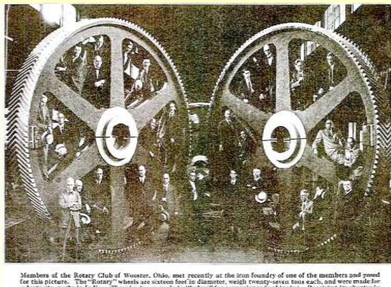
Members of the Rotary Club of Wooster, Ohio, met recently at the iron foundry of one of the members and posed for this picture. The "Rotary" wheels are sixteen feet in diameter, weigh twenty-seven tons each, and were made for a large cin works in India. The wheels are made in "halves" for convenience in shipping. Receiving its charter in
